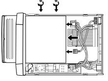
$Step 11 \overset{\text{Secure the bondi cover into place with the}}{{}_{two \ screws \ and \ your \ CD-ROM/ \ RW}}$ ready to go!
