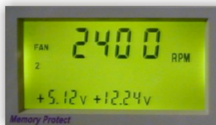
Fig.3 LCD Display - Back-light On - Scan Mode
